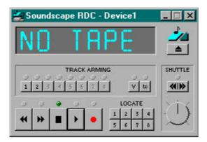
Soundscape has a software **Remote Device Control (RDC)** for the DVCPRO source machine, usually situated at the bottom right of the screen. When recording back on to tape you MUST use the RDC to avoid erasing your visuals!
